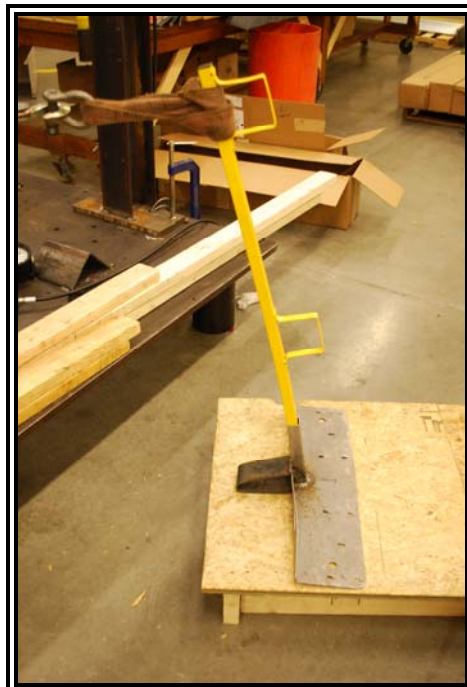
Figure 2: Stand-alone setup without handrail with load applied
